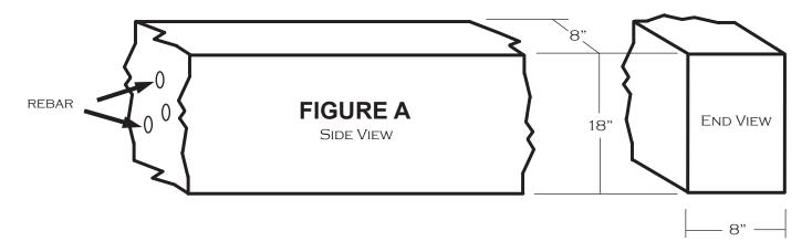
1 CUBIC YARD OF CONCRETE = 27 CUBIC FEET OR EQUIVALENT OF 27 LINEAL FEET (EACH LINEAL FOOT OF FOOTING SHOWN IN FIGURE A EQUALS 1 CUBIC FOOT)
